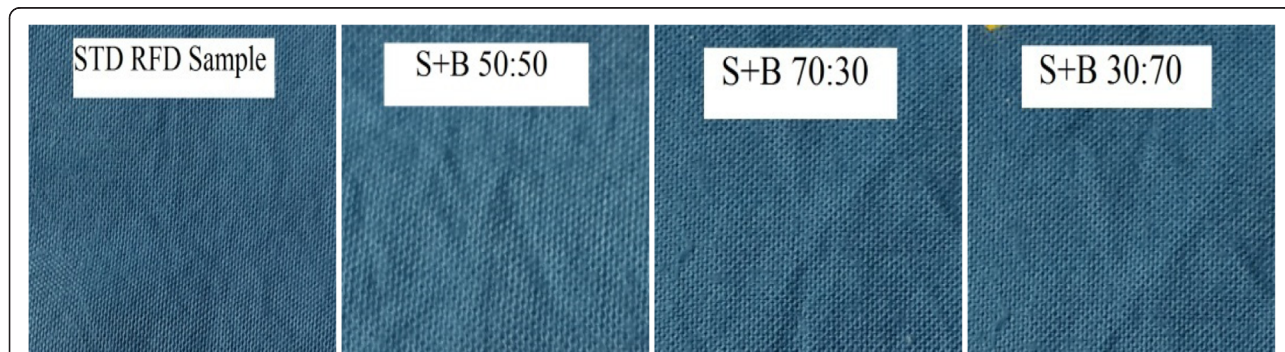
Fig. 5 Samples dyed using Navy Blue HER. First sample is a standard ready for dyeing (RFD) fabric dyed with Navy Blue HER, second, third and fourth dyed ones are grey fabrics desized using scouring to bleaching wastewater in 50:50, 70:30 and 30:70 ratios, respectively
