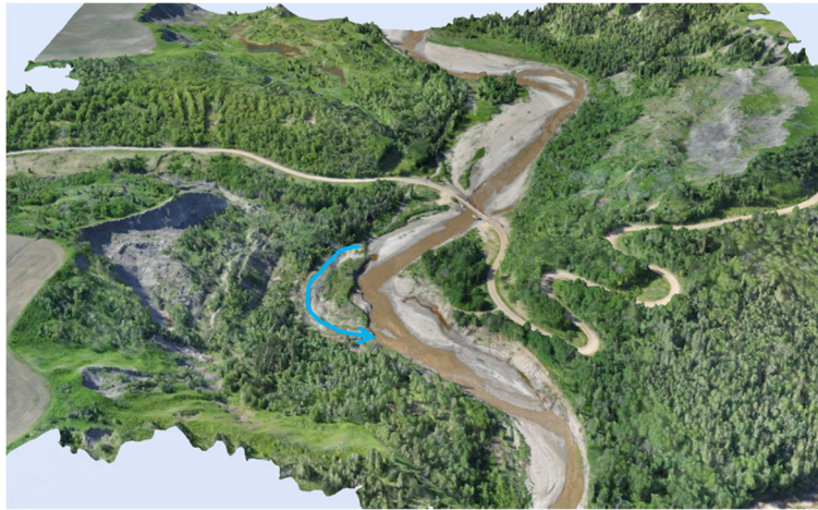
Fig. 10 Oblique aerial image mosaic of drone imagery, from June 2017, draped over a photogrammetrically generated digital elevation model depicting the Pouce Coupe River, and Landry Road and bridge (Source: Government of British Columbia; reproduced with permission). The 2013 landslide and dam are visible in the lower left. The approximate trace of the pre-landslide Pouce Coupe River channel is the blue line. The post-landslide stream channel cut through a point bar attached to the opposite stream bank, abandoning the pre-landslide channel
