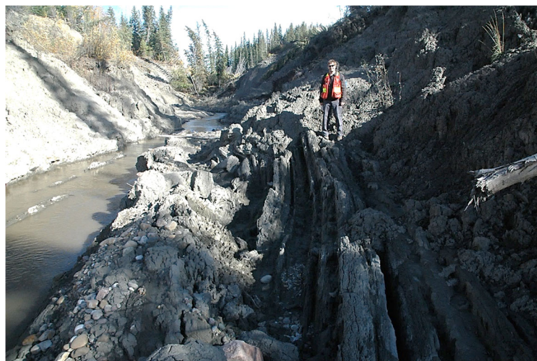
Fig. 3 Upthrust advance phase glacial lacustrine sediment (LTA3) at the toe of the Eureka River landslide. The reorientation of the lacustrine rhythmites to near vertical, was likely caused by the landslide. Note the scattering of boulders and cobbles at discrete locations. This material likely originated in the pre-landslide channel and was introduced into the post-landslide channel by bank erosion. Also note the small landslide into the channel in the distance. (Source: BGN Miller, September 28, 2007)
