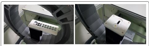
**Fig. 6** Left, photograph of the holder and source used for the spatial resolution studies along the radial axis. Right, holder for the sensitivity measurements
