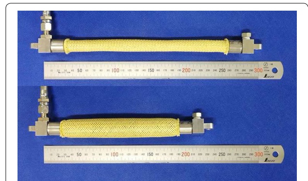
Fig. 1 Photo of the HAM used in this study in rest state and contracted state with 3 MPa applied pressure
