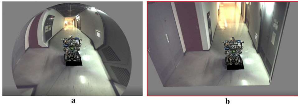
Fig. 12 Free viewpoint image generation in a corridor. a Generated by the previous method [7]. b Generated by the proposed method. The previous method generated distorted free viewpoint images, which makes it more difficult for operators to perceive the distance between the robot and the walls. On the other hand, the distance between the robot and the walls is obvious in images generated by the proposed method
