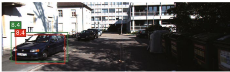
Fig. 2 Examples of the relation between the appearance of target objects (cars), and those distance in KITTI dataset. The green and red rectangles are the ground truth and estimated bounding boxes (by our proposed method) respectively. The values in green and red boxes are the GT and estimated distances respectively in a meter. The distance of the car on the left-hand side is 8.4 m
