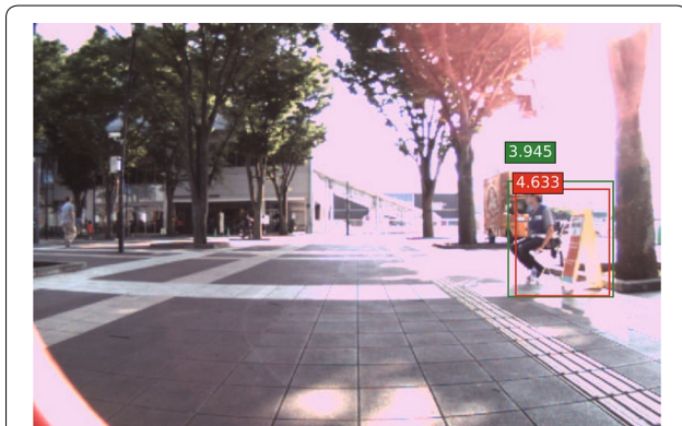
Fig. 18 Examples of estimated distance for the side-view of the target object in Tsukuba Challenge. The ground truth distance and estimated distance are written in green and red boxes respectively. The unit is in meter
