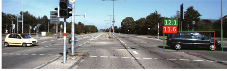
Fig. 1 Examples of the relation between the appearance of target objects (cars), and those distance in KITTI dataset. The green and red rectangles are the ground truth (GT) and estimated bounding boxes (by our proposed method) respectively. The values in green and red boxes are the GT and estimated distances respectively in meter. The distance of the car on the right hand side is 12.1 m
