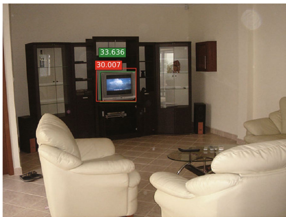
Fig. 11 Examples of results in Pascal3D+ TV monitor for a medium size TV monitor. The ground truth distance and estimated distance are written in green and red boxes respectively. The unit of distance is based on CAD models
