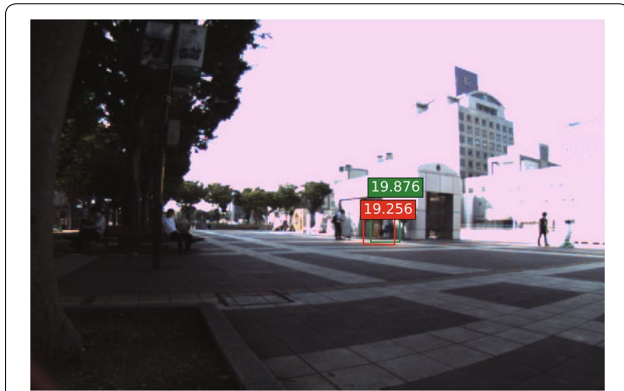
Fig. 20 Examples of estimated distance for the far-view of the target object in Tsukuba Challenge. The ground truth distance and estimated distance are written in green and red boxes respectively. The unit is in meter
