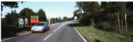
Fig. 3 Examples of the relation between the appearance of target objects (cars), and those distance in KITTI dataset. The green and red rectangles are the ground truth and estimated bounding boxes (by our proposed method) respectively. The values in green and red boxes are the GT and estimated distances respectively in a meter. The distance of the car on the left-hand side is 11.9 m
