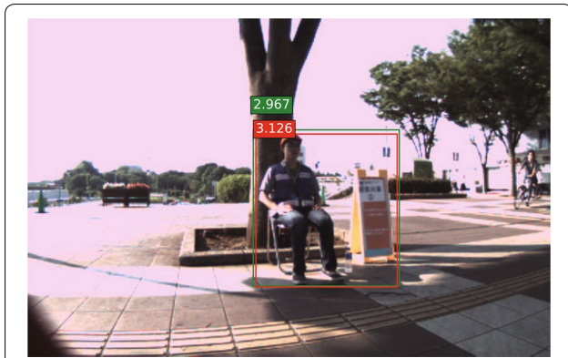
Fig. 19 Examples of estimated distance for the front-view of the target object in Tsukuba Challenge. The ground truth distance and estimated distance are written in green and red boxes respectively. The unit is in meter
