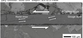
**Fig. 7** Back-scattered electron images of the recovered samples **A** C0002N-141SW and **B** C0002P-266SW. The gouge layer is sandwiched between the gabbro forcing blocks, and the arrows in the blocks indicate slip directions. Riedel shears are widely developed in these samples. These images were taken using an electron-probe microanalyzer with a 15-kV accelerating voltage and 2.5 nA probe current
