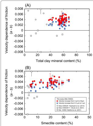
**Fig. 9** Relationship between a-b and **A** total clay mineral content and **B** smectite content. Red and blue circles indicate the results for velocity change from 3 to 33  $\mu$ m/s and from 0.3 to 3  $\mu$ m/s, respectively. Open circles, squares, and diamond indicate data from previous studies of the Nankai samples along the Kumano transect (Takahashi et al. 2014; Okuda et al. 2021; Bedford et al. 2021)
