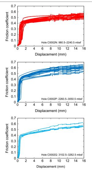
**Fig. 4** Results of the frictional experiments of the cuttings samples collected from Holes C0002N (980.5–2240.5 mbsf), C0002P (2260.5–3050.5 mbsf), and C0002Q (3102.5–3262.5 mbsf). The experiments were run at a slip velocity of 3  $\mu$ m/s for the first 8 mm of displacement, followed by stepwise changes of 0.3, 3, and 33  $\mu$ m/s to test the velocity dependence of friction
