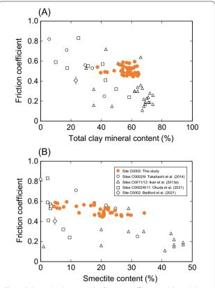
**Fig. 8** Relationship between the friction coefficient and **A** total clay mineral content and **B** smectite content. Data obtained in this study are shown by orange circles, and open circles, triangles, squares, and diamond indicate data from previous studies of the Nankai samples collected along the Kumano transect (Takahashi et al. 2014; Ikari et al. 2013a; Okuda et al. 2021; Bedford et al. 2021)
