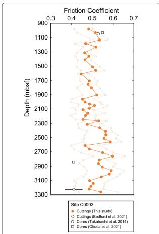
**Fig. 5** Depth profile of the friction coefficient obtained via analysis of the cuttings at Site C0002. Friction coefficient obtained at a displacement of 8 mm is shown by orange filled circles, and the lower and upper data (orange open circle) are obtained at displacements of 2 mm and 16 mm, respectively. The black open circles, squares, and diamond indicate data from previous studies at Site C0002 (Takahashi et al. 2014; Okuda et al. 2021) Bedford et al. 2021)
