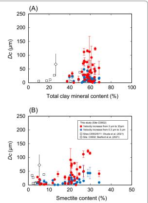
**Fig. 10** Relationship between  $D_c$  and **A** total clay mineral content and **B** smectite content. Red and blue circles indicate the results for velocity change from 3 to 33  $\mu$ m/s and from 0.3 to 3  $\mu$ m/s, respectively. Open squares and diamond indicate data from previous studies of the Nankai samples along the Kumano transect (Okuda et al. 2021; Bedford et al. 2021)
