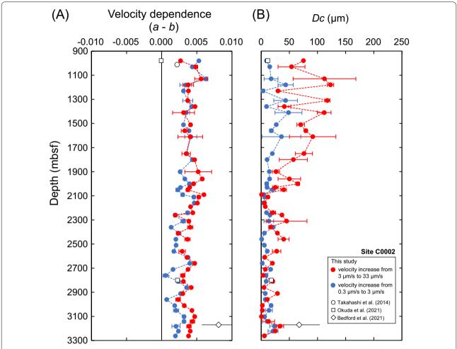
**Fig. 6** Depth profiles of **A** the velocity dependence of friction a-b and **B** critical slip distance  $D_c$  at Site C0002. Red and blue circles indicate the results for velocity change from 3 to 33  $\mu$ m/s and from 0.3 to 3  $\mu$ m/s, respectively. The error bars are estimated from the variations in the repeated tests. Open circles, squares, and diamond indicate data from previous studies at Site C0002 (Takahashi et al. 2014; Okuda et al. 2021; Bedford et al. 2021)
