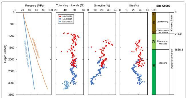
**Fig. 2** Pressure, clay mineral content, and unit classification profiles for Site C0002 (after Tobin et al. 2015, 2020; Underwood 2017a, b; Kitajima et al. 2020). The lithospheric pressure is calculated from the overburden stress, which is derived from the rock density, and the hydrostatic pore pressure is calculated using a fluid density of 1.024 g/cm<sup>3</sup>
