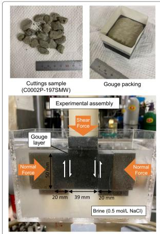
**Fig. 3** Photographs of the cutting samples, preparation of the simulated gouges, and experimental apparatus. The experiments were conducted under fluid-saturated conditions using a 0.5 mol/L NaCl solution
