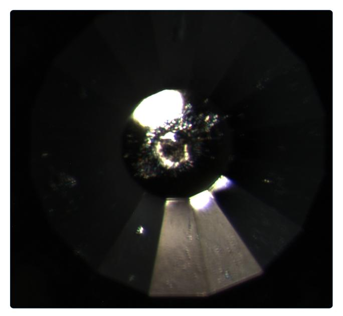
Unit cell determination of coexisting post-perovskite and H-phase in (Mg,Fe)SiO<sub>3</sub> using multigrain XRD: compositional variation across a laser heating spot at 119 GPa
