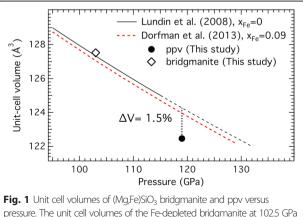
pressure. The unit cell volumes of the Fe-depleted bridgmanite at 102.5 GPa and the ppv phase at 119 GPa coexisting with the H-phase are compared with the equations of state for Fe-free MgSiO<sub>3</sub> bridgmanite (Lundin et al. 2008) and (Mg<sub>0.91</sub>Fe<sub>0.05</sub>)SiO<sub>3</sub> bridgmanite (Dorfman et al. 2013)
