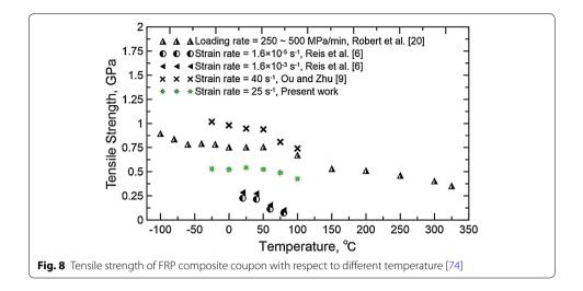
Many researchers shows an improved strength of FRP composites at low temperature and a possible explanation for improved strength is FRP matrix embrittlement and matrix hardening [84–87]. The composite behavior at low temperatures depends to a large degree on the type of polymer matrix and its sub-zero mechanical properties.
