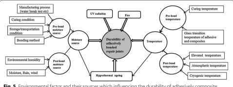
**Fig. 5** Environmental factor and their sources which influencing the durability of adhesively composite bonded joints
