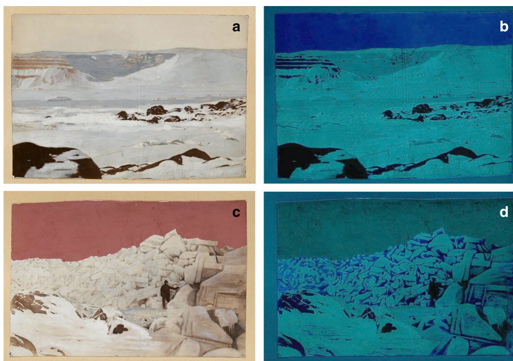
Fig. 5 Normal light (left) and UV light (right) photographs of a, b plate 11 and c, d plate 23 (improved positives). The intense yellow fluorescence detected in areas retouched with white overpaint suggests the use of a zinc oxide pigment
