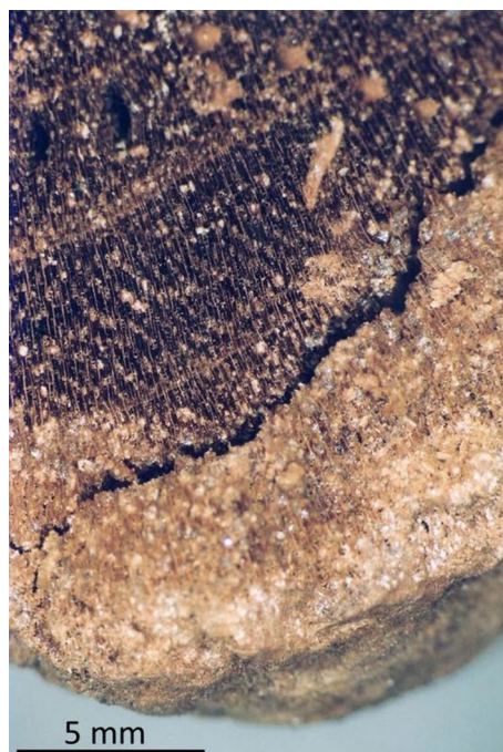
Fig. 4 Stereomicroscope image of alum crystals in wood. The crack has formed along the alum-rich and alum-poor boundary. Photo: SB
