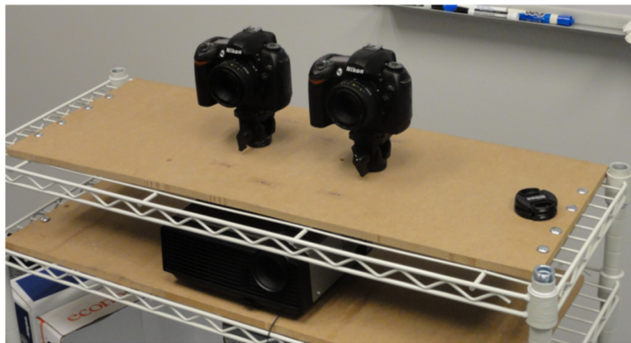
Figure 2 Our stereoscopic system. Our stereoscopic system is made up of two D70s Nikon cameras, a high-resolution video projector, and a laptop.
