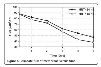
The fouling is the major problem with membranes in separation processes. Nevertheless, RBC was used as a pre-treatment stage and the most of the wastewater was treated before entering into the membrane which results in the reduction of the fouling. Membrane fouling in this study took place after 120 hours from the beginning and after cleaning the membrane was reutilized. This is more than the time needed in previous studies [14].
