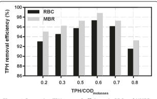
Figure 4 Comparing TPH removal efficiency in RBC and HMBR in different ratios of TPH/COD molasses at HRT of 24 hours.
