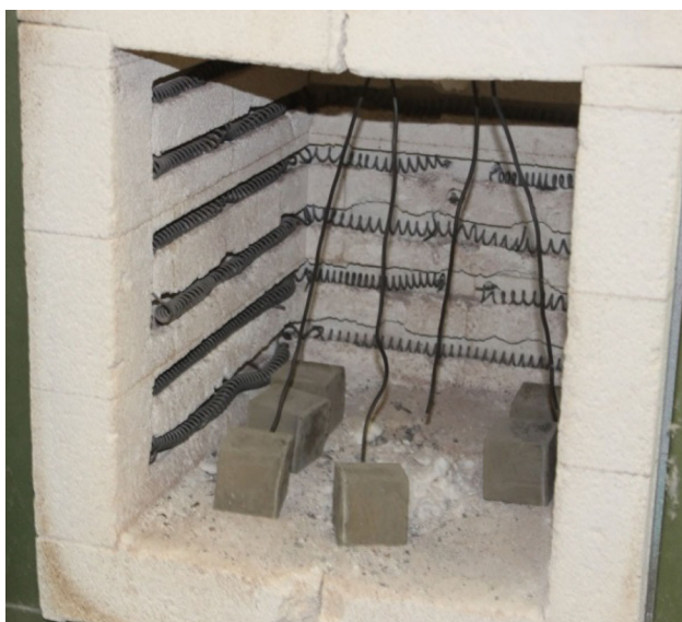
Fig. 1 Locally manufactured kiln to heat the geopolymer composite specimens at various elevated temperatures.
