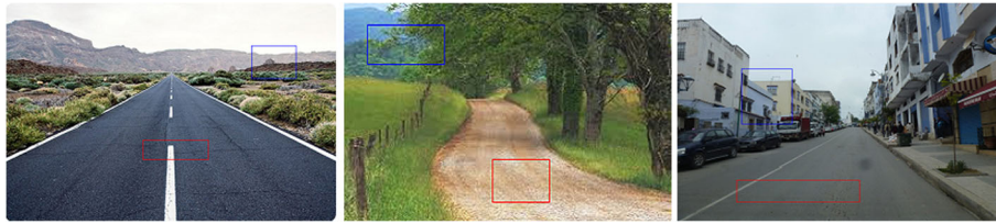
Fig. 3 Initialization of DTD. Red rectangles are used for “positive” training (road class), and blue ones for “negative” training (non-road class)
