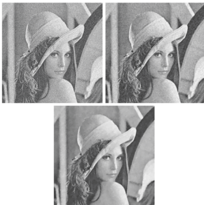
Fig. 2 Denoising of the Lena image using different methods. Top left : a noisy image with Gaussian noise ( \sigma = 15 ). Top right : the denoised image by CEP- L_2 with PSNR = 29.7321. Bottom : by NLCEP- L_2 with PSNR = 30.8995
