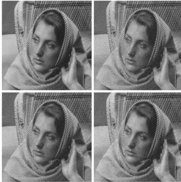
Fig. 4 Denoising of the Woman image using different methods. Top left : the original image. Top right : a noisy image with Gaussian noise ( \sigma = 10 ). Bottom left : the denoised image by CEP- L_2 with PSNR = 29.0179. Bottom right : by NLCEP- L_2 with PSNR = 29.2275
