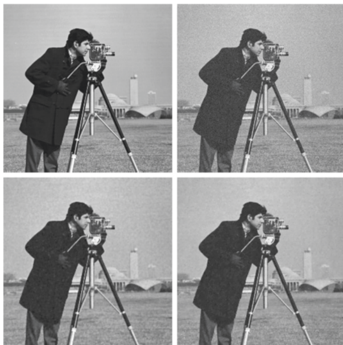
Fig. 3 Denoising of the Cameraman image using different methods. Top left : the original image. Top right : a noisy image with Gaussian noise ( \sigma = 10 ). Bottom left : the denoised image by CEP- L_2 with PSNR = 31.4397. Bottom right : by NLCEP- L_2 with PSNR = 32.3308
