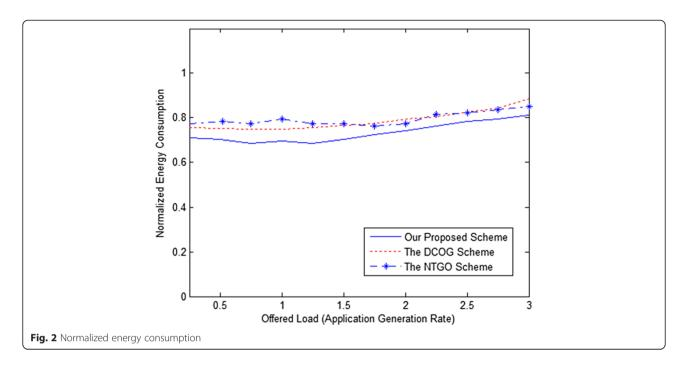
our nested game model could lead to higher energy efficiency than the *DCOG* and *NTGO* schemes. When designing an effective computation offloading scheme, it is a highly desirable property.
