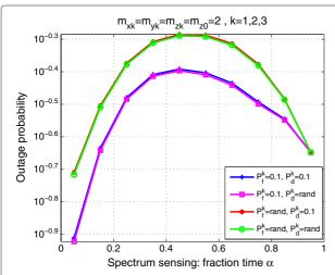
**Figure 5** Outage probability versus spectrum sensing overhead  $\alpha$  for a fixed/random values of the probabilities of false alarm and of detection.
