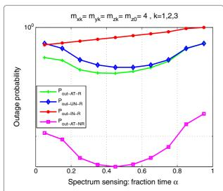
**Figure 8** The outage probability of different strategies of transmission under a poor fading and a random average channel gain.
