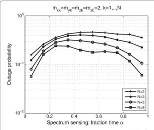
**Figure 4** Outage probability versus spectrum sensing overhead  $\alpha$  for different values of the number of relay N.
