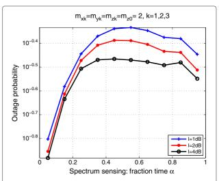
**Figure 3** Outage probability versus spectrum sensing overhead  $\alpha$  for different values of the interference power constraint *l*.
