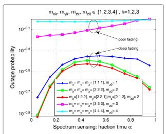
**Figure 6** Outage probability versus spectrum sensing overhead  $\alpha$  for different values of the fading severity parameters  $(m_{xk}, m_{yk}, m_{zk}, m_{z0}, k=1,2,3)$ .
