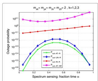
**Figure 7** The outage probability of different strategies of transmission under a deep fading and a random average channel gain.
