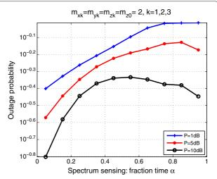
**Figure 2** Outage probability versus spectrum sensing overhead  $\alpha$  for different values of the transmission power P at (CS and  $CR_k$ ).
