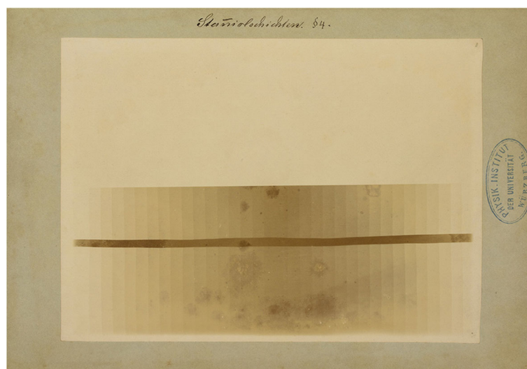
Fig. 5 Stacks of tin foil with various thicknesses. This image shows that the thicker the stack, the less X-radiation passes through it. Manually written legend: 'Stanniolschichten' (Layers of tin foil). Paragraph referral: § 4
