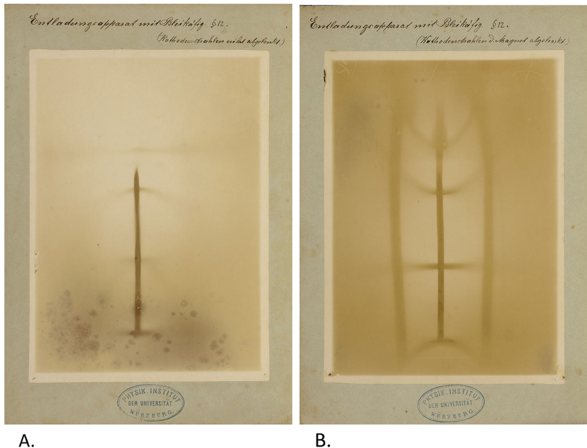
Fig. 8 a, b Two radiographic images of a leaden cage that surrounds the gas discharge tube. The difference between them is that the second image was taken while the cathode rays were deflected using a magnet while in the first image the magnet was absent. Between the two radiographs, the shadow of the leaden cage moved. Roentgen concluded from this that the X-rays had to emanate from the point on the glass wall of the discharge tube where the cathode rays impinged and this point had moved as a result of the deflection of these cathode rays. It can be noticed that the magnet pulls the focal spot downward, resulting in the central ray to hit the center of the cage (shadow of the ribs at the top of the cage bend upward and the brightest part of the background moves downward) while, at the same time, the focal spot becomes smaller (image becomes sharper). Respective manually written legends: 'Entladungsapparat mit Bleikäfig (Kathodenstrahlen nicht abgelenkt)' (Gas discharge tube with leaden cage (cathode rays not deflected)) and 'Entladungsapparat mit Bleikäfig (Kathodenstrahlen durch Magnet abgelenkt)' (The word 'durch' was completed by the author) Magnet abgelenkt' (Gas discharge tube with leaden cage (cathode rays deflected by a magnet)). Paragraph referral: § 12 (in both radiographs)
