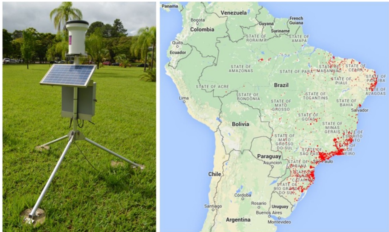
Fig. 1 DCP and network geographical coverage. (Left) Photo showing an autonomous DCP type unit called pluvio containing the rain gauge, solar panel, GSM/3G antenna, and the electronic control box mounted on an aluminium frame. A high-gain antenna provides GSM/GPRS link to a distant radio base station. (Right) 2015 CEMADEN network of pluviometric DCPs (red dots) installed on the Brazilian territory
