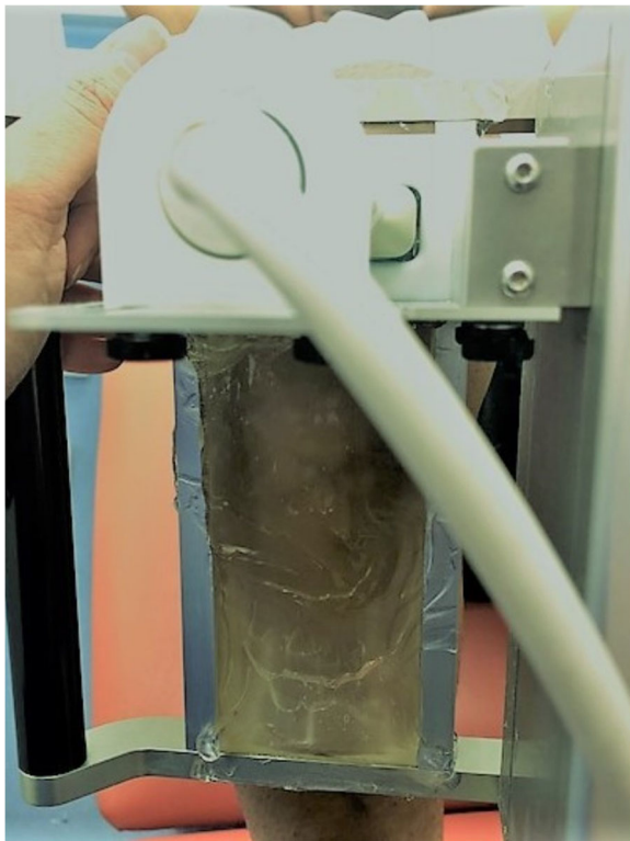
Fig. 1 Superior view of UTC transducer transversely fixed into tracking device for scanning a right patellar tendon
