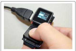
**Fig. 1** Photograph of the developed device. The feedback function is shown in an OLED display
