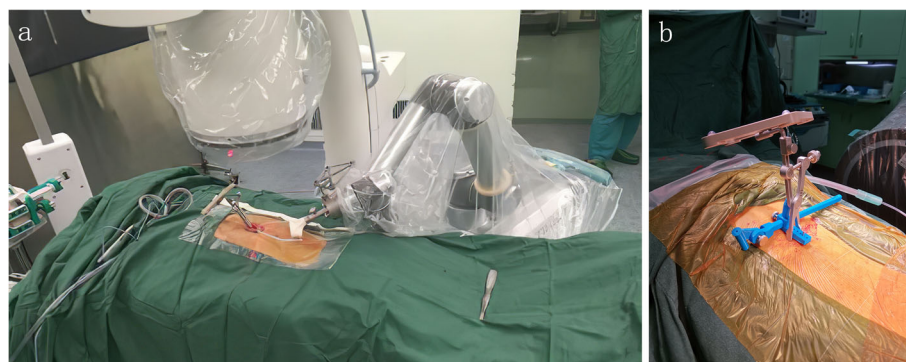
Fig. 1 The base of the tracer in Tirobot system. a Traditional tracer base. b Self-made tracer base
