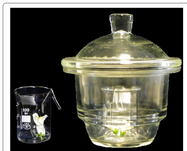
Fig. 1 Sampling system for VOCs in HSSE
