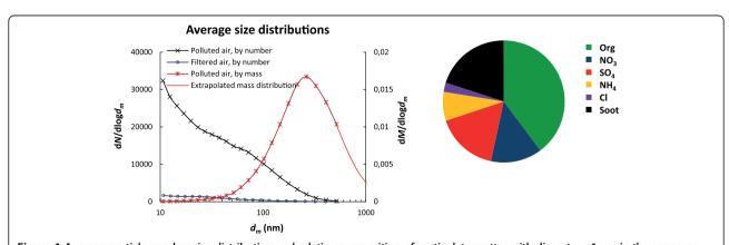
Figure 1 Average particle number size distribution and relative composition of particulate matter with diameter <1 µm in the exposure chamber assessed by a Scanning Mobility Particle Sizer, a Differential Mobility Analyzer coupled in series with an Aerosol Particle Mass Analyzer and an Aerosol Mass Spectrometer.
