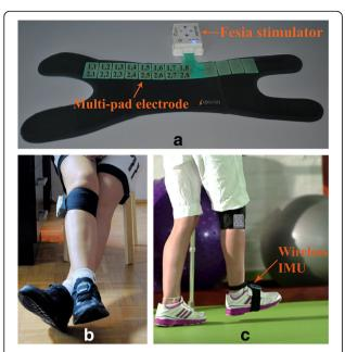
**Fig. 1** Fesia Walk system (Tecnalia R&I, Donostia/San Sebastián, Spain). **a** Electrical stimulator and multi-pad electrode with physical coordinates attached to the garment. **b** Position of a patient during setup process. **c** FES-assisted gait
