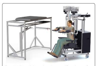
**Fig. 1** KINARM exoskeleton robotic device used for evaluation of motor and proprioceptive deficits of subjects with stroke
