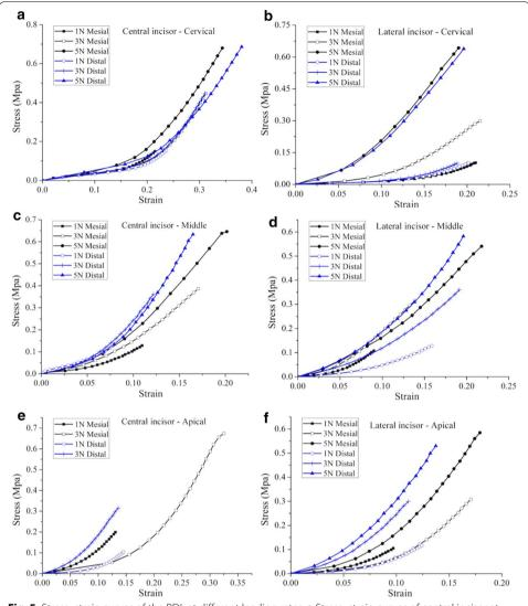
**Fig. 5** Stress–strain curves of the PDL at different loading rates. **a** Stress–strain curves of central incisor at cervical level; **b** stress–strain curves of lateral incisor at cervical level; **c** stress–strain curves of central incisor at middle level; **d** stress–strain curves of lateral incisor at middle level; **f** stress–strain curves of lateral incisor at root level; **f** stress–strain curves of lateral incisor at root level
