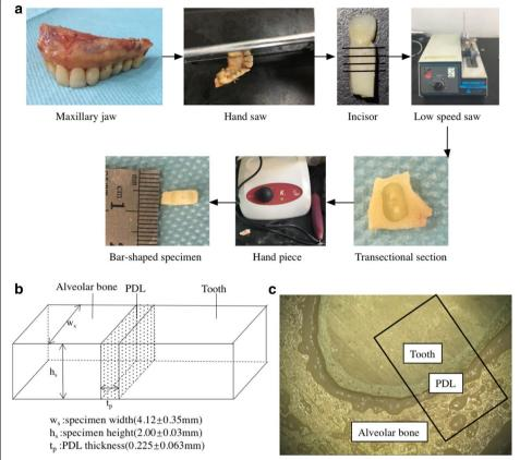
**Fig. 2** The specimen preparation process. **a** The procedure begins with human maxilla used to form bar-shaped specimens, **b** dimensions of the PDL specimens, **c** photo of bone–PDL–tooth complex under stereomicroscope
