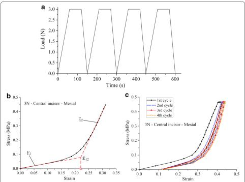
**Fig. 4** Loading cycles and stress–strain curves of the load case with 3 N force amplitude. **a** Loading cycles in the uniaxial tensile test, **b** illustration of the procedures for determining  $E_1$ ,  $E_2$  and  $\epsilon_{12}$  of the bilinear elastic model, **c** stress–strain curves of the PDL for four loading cycles
