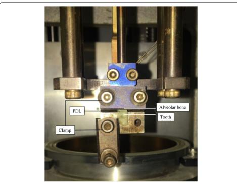
Fig. 3 Specimens fixed by the clamps of the DMA equipment
