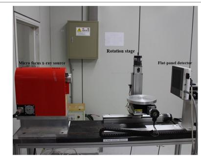
Fig. 5 The lab-built micro-CT system consisting of a micro-focus x-ray source, a flat-panel detector and a rotating stage
