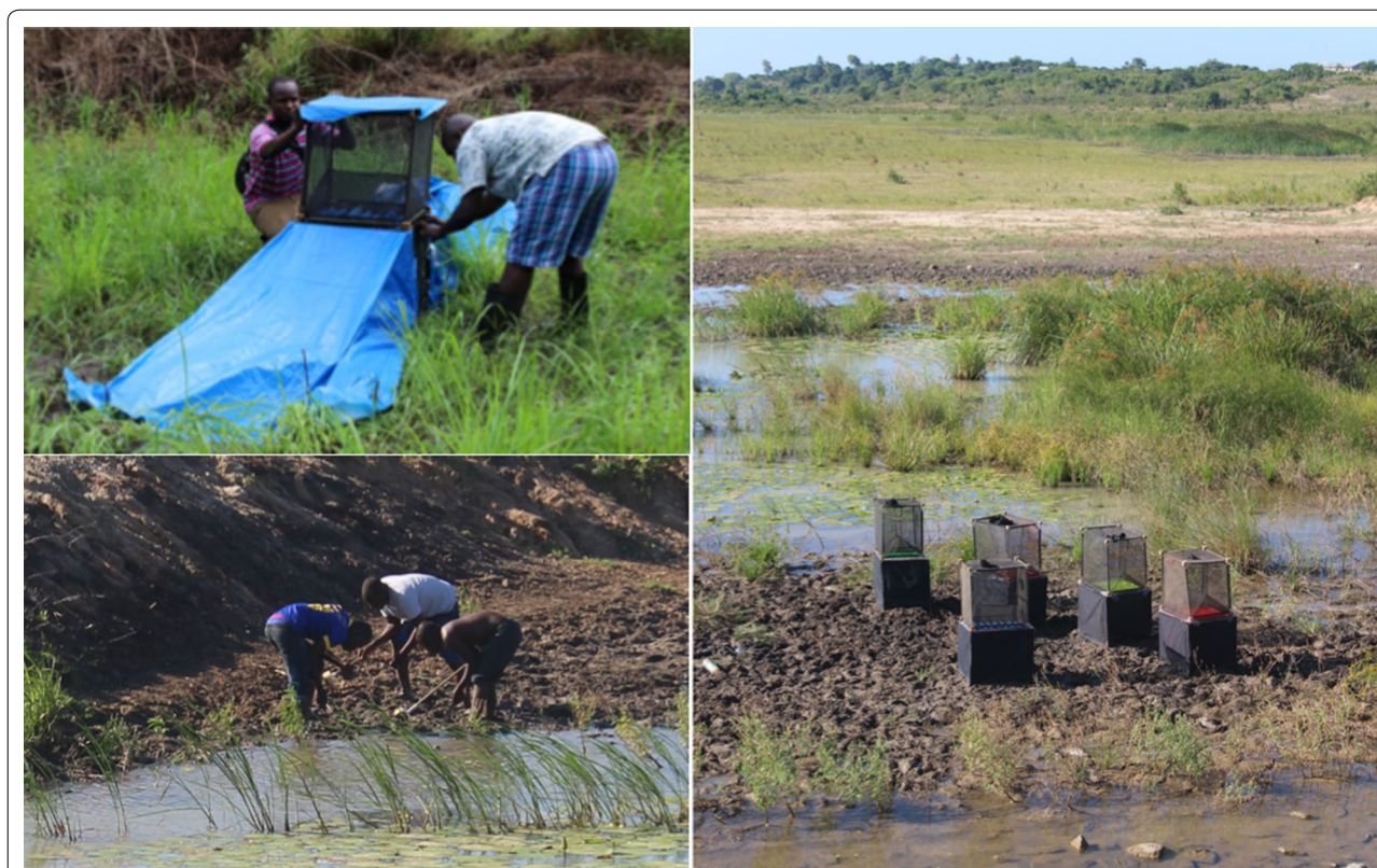
Fig. 4 Self-marking units in the field with exit traps to measure exiting rates of mosquitoes from natural breeding sites and sites where the numbers of pupae were manipulated. Top left: self-marking UNIT with tarpaulin skirt extension to cover a ditch where Anopheles larvae were found. Right: five basic self-marking units containing the five pigments used in the study (pink, orange, yellow, green and blue). Bottom left: pupae collection with dippers. Larval dippers were first used to identify productive breeding sites and then to collect pupae to be placed under the self-marking devices
