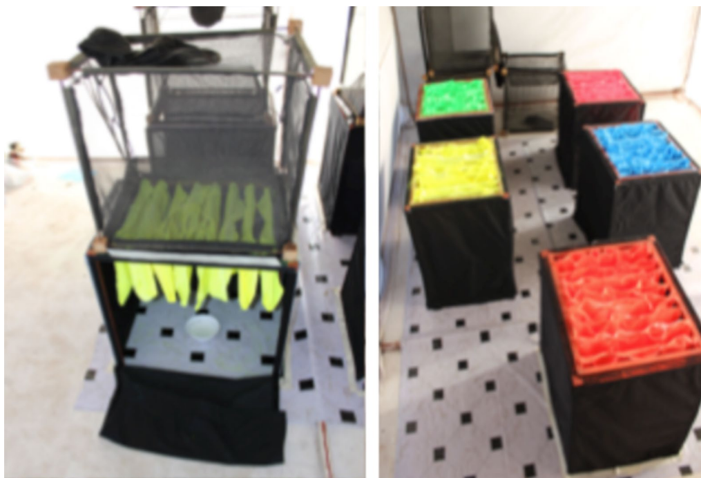
Fig. 3 Evaluation of the self-marking units under semi-field conditions. Left panel: an open side panel showing a bowl of An. arabiensis pupae underneath. The side panel is closed for the experiment and emerging adult mosquitoes fly and bump their way through the layers of cloth to exit the marking grid and into the exit trap. Adults are collected from the exit trap by aspiration through the cloth sleeve on top of the trap. Right panel: the units set-up as intended for field use with side panels closed and exit traps removed. Five units each containing a different colour marker used in the study
