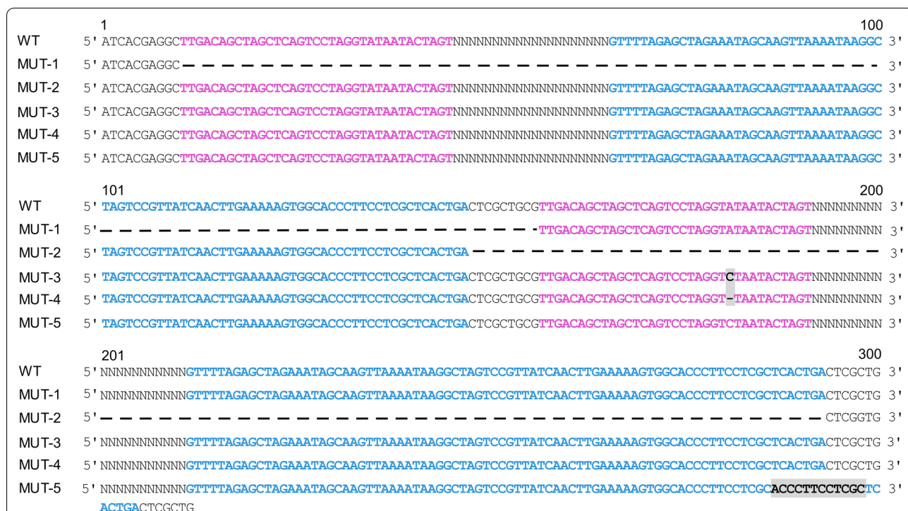
Fig. 2 Representative DNA sequencing results of recombination derivatives from pDG-A-X series. MUT-1 had deletion of the first gRNA expression cassette; MUT-2 had deletion of the second gRNA expression cassette; MUT-3 and MUT-4 had point mutations in the second promoter J23119; MUT-5 had 12-bp repeated insertion in the second gRNA scaffold. Promoter J23119 (purple), 82-bp scaffold (blue) and the mutated sequence (highlighted) are denoted. The strikeout represents deleted sequence
