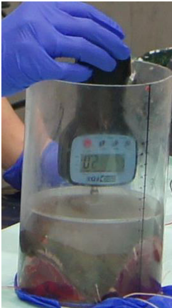
Fig. 5 Pressure application with the algometer to the middle of a back tissue section
