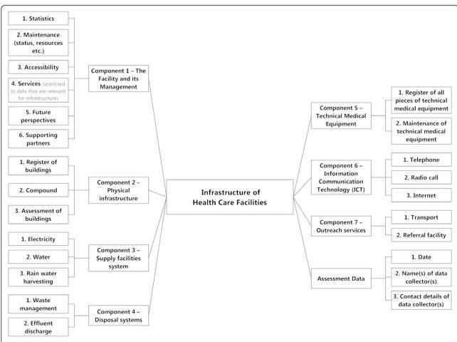
**Figure 2** Aspects of facility infrastructure assessment. Figure 2 shows details of facility infrastructure assessment which describe aspects under the seven major components (compare figure 1).
