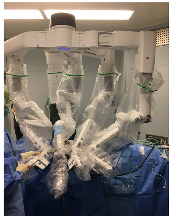
Fig. 6 Docking: Da Vinci Xi docked in position with four arms engaged
