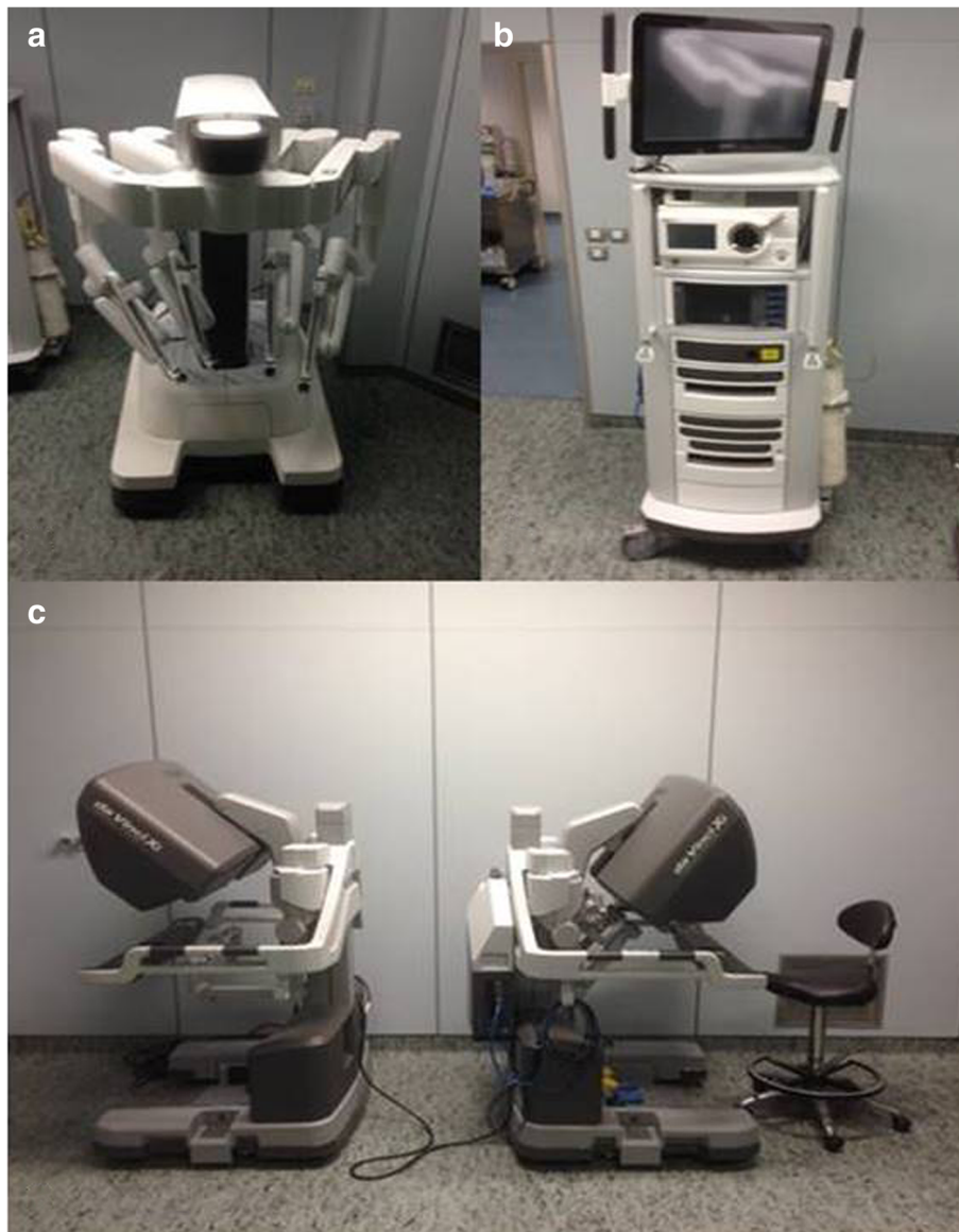
Fig. 2 Da Vinci Xi Surgical System (Intuitive Surgical Inc., Sunnyvale, CA, USA): a Patient cart; b Da Vinci Surgical System Xi: Video cart; c Da Vinci Surgical System Xi: Surgeon console
