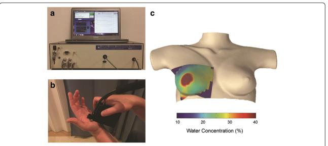
Fig. 2 Diffuse Optical Spectroscopic Imaging (DOSI): a Portable, bedside DOSI instrument, b Handheld DOSI probe that is scanned across the breast to collect data, and c DOSI image of breast water concentration
