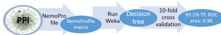
Fig. 9 Process to predict essential proteins in a PPI network. A PPI network is processed to obtain NemoProfile matrix ( A ) that shows protein i has A_{ij} overlaps with motif j . The matrix is directly loaded into a Weka program to run a decision tree algorithm and is evaluated through 10-fold cross-validation method to provide prediction rate and ROC area value as a result
