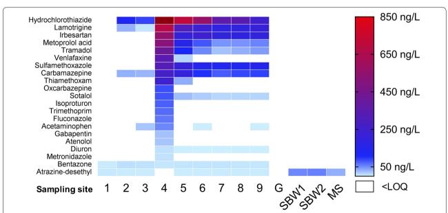
**Fig. 2** Detected target pollutants from sampling sites 1 to 9 along the Ammer River, the tributaries Schönbrunnen (SB) and Mühlbach (MS) and from one sample of the Kleiner Goldersbach (G) creek. The concentration of hydrochlorothiazide at site 4 was 1.9  $\mu$ g L<sup>-1</sup> which exceeds the concentration scale and is colored in dark red
