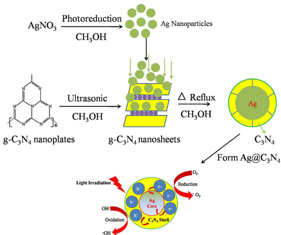
Fig. 10 Schematic drawing illustrating synthetic route (templating method) and the mechanism of charge separation and photocatalytic process over C 3 N 4 and Ag@C 3 N 4 photocatalysts under light irradiation. Reproduced with permission [124]. Copyright 2014 Elsevier.
