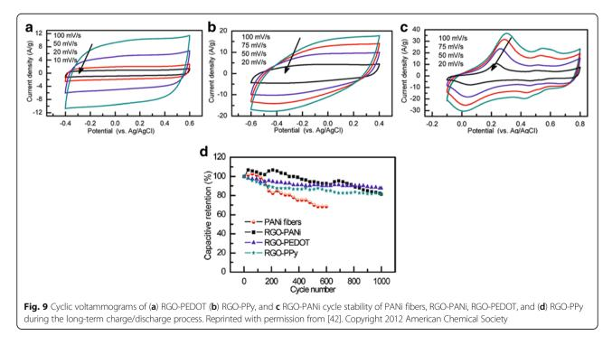
addition, all the composite supercapacitor electrodes showed good cycling performance compared to pristine PANI fibers with capacitance retention of only 68% after 600 cycles. However, RGO/PEDOT has the best capacitance retention of 88% after 1000 cycles, while RGO/ PANI and RGO/PPy have the similar cycling performance of 82 and 81% retention after 1000 cycles [42].
