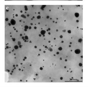
Figure 3 Representative TEM images of AuNPs obtained under different conditions. (a) 40 mL IPE, 1.0 mM, pH = 2.7. (b) 80 mL IPE, 1.5 mM, pH = 2.5. (c) 80 mL IPE, 1.0 mM, pH = 4.0.
