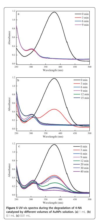
AuNPs and protein extract by functional groups including hydroxyl, amine, and carboxyl, which were possibly responsible for the reduction of gold ions and stabilization. The biosynthesized AuNPs could effectively catalyze the degradation of 4-NA, and 0.019 mg of AuNPs with average size of 6.07 nm was optimized to completely degrade 12.5  $\mu$ mol of 4-NA in 6 min. It was
