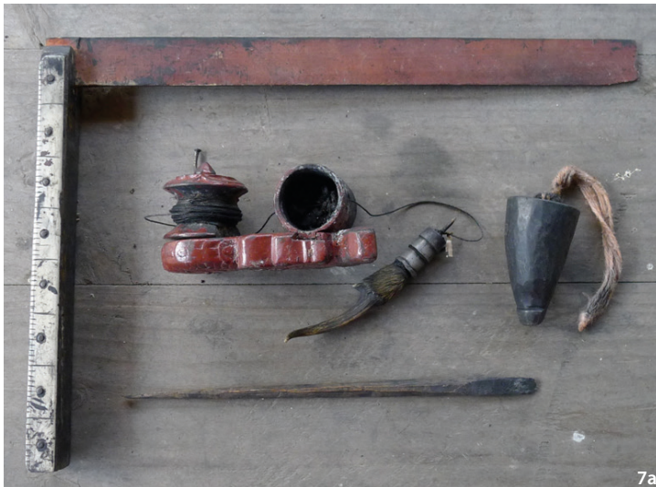
Figure 7a Tools used for the mark-ink work (Source: Congcong Ren).
