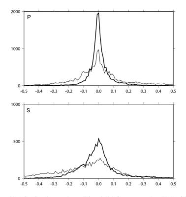
Fig. 3. The frequencies of the residuals for all stations are shown. Thin and thick lines represent the residuals of the initial and final frequencies, respectively. At the end of this analysis, the averaged residual of hypocenter determination decreased from 0.131 to 0.054 s for P-wave arrival and from 0.193 to 0.100 s for S-wave arrival. Note that the shape of the curve of frequency becomes sharp.
