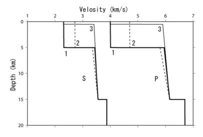
Fig. 2. P-wave and S-wave velocity structure models for hypocenter determination. These models were derived from previous refraction experiments (Imai *et al.*, 2004; Takeda *et al.*, 2004). Model numbers 1 (thick line), 2 (broken line) and 3 (thin line) were adapted for the regions around the ISTL (1, 2, 6 and 8 in Fig. 1), for the south-east region (9) and for the other regions (3, 4, 5 and 7), respectively.
