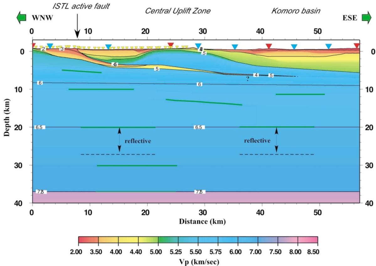
Fig. 2. P-wave velocity structure by ray-tracing method along Itoshizu 2002 seismic line (Sato *et al.*, 2004a) after Imai *et al.* (2004). Red triangles: locations of explosive sources, blue triangles: locations of high energy shots (a large number of sweeps) by vibroseis trucks, yellow triangles: locations of vibroseis shot points used in this analysis. Green lines represent the reflectors clearly observed on the shot gathers by explosive sources.
