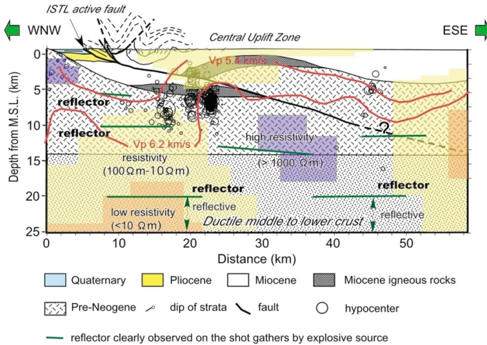
Fig. 5. Geologic cross-section along the Itoshizu 2002 seismic line (Sato *et al.*, 2004a) with the resistivity structure (Ogawa *et al.*, 2002), the hypocentral distribution (Sakai, 2004) and P-wave velocity structure obtained by seismic tomography (Kurashimo and Hirata, 2004). The location of deep reflectors is after Imai *et al.* (2004).
