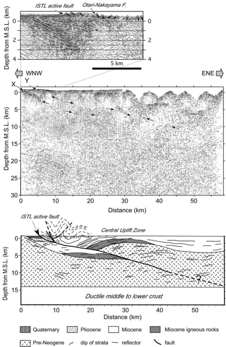
Fig. 3. Stacked, migrated, depth converted seismic sections of Itoshizu 2002 and its geologic interpretation after Sato *et al.* (2004a). X: base of Neogene, Y: deeper extension of the ISTL active fault.
