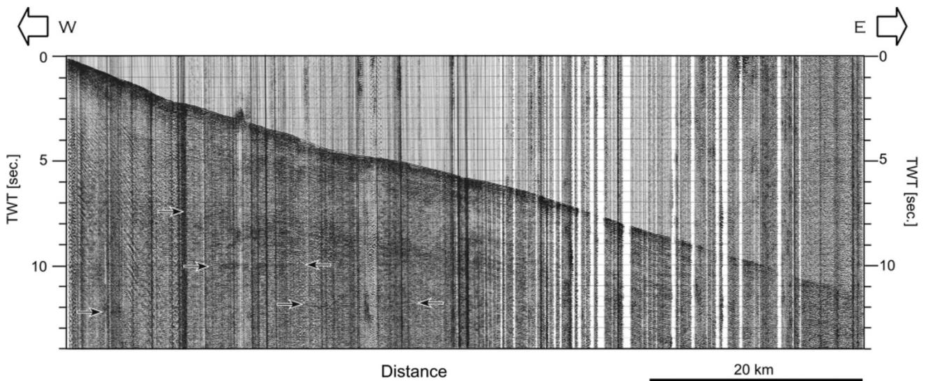
Fig. 4. Shot record by explosive source (100 kg of dynamite) at the western end of the Itoshizu 2002 seismic line. Arrows indicate the significant reflection from middle to lower crust.
