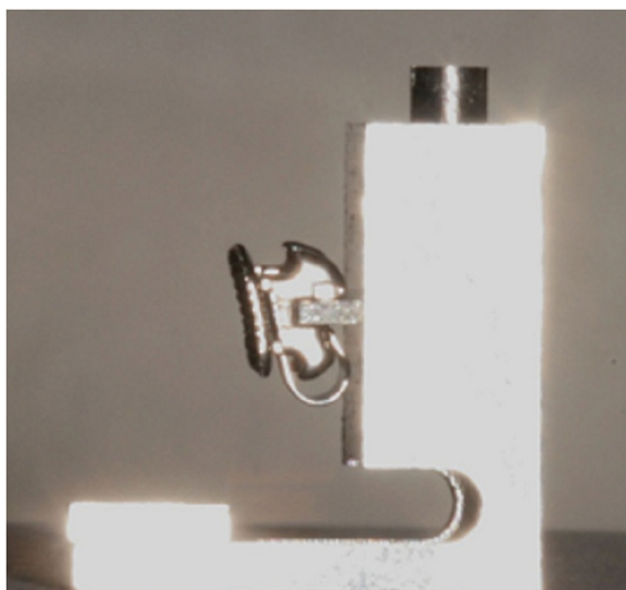
Figure 1 L-shaped FAQ.FIX® prototype with horizontal and vertical arms and insert for the slot reproducing bracket angulation.
