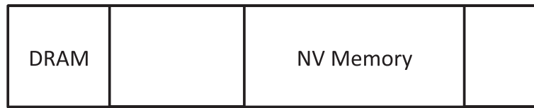
Figure 3 Physical address space of the target system.
