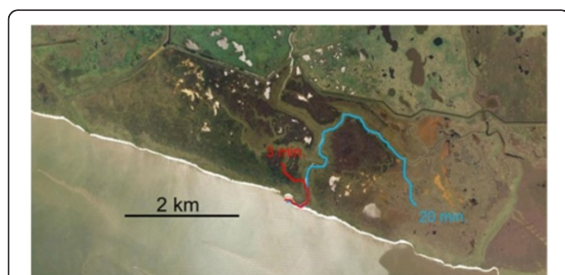
Figure 2 Two examples of water paths in a salt marsh, computed on the basis of water surface gradients (e.g., Rinaldo et al. 1999), and related travelling times. During flood, the water moves first in the channels and then on the marsh surface. The travelling times for all marsh locations need to be computed in order to determine the distribution f .
