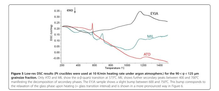
samples and not in the composition alone. The glass transition peak is less pronounced than for pure glasses; we relate this to the presence of crystals in the glass and a distribution of iron in different oxidation states (Kremers et al. 2012).
