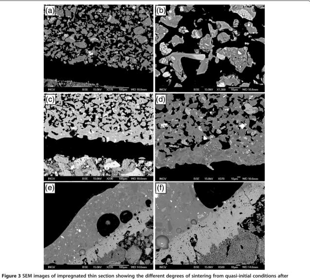
60 minutes at 950°C (a overview, b detail), through considerable neck formation after 60 minutes at 1000°C (c overview, d detail) to complete textural densification after 60 minutes at 1050°C (e overview, f detail).
