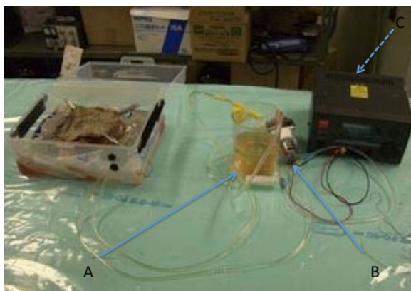
Figure 1 The cryopreserved kidney is perfused by a peristaltic pump after thawing, and contained entirely in a “Bento” lunchbox. (A = Fluid reservoir, B = Peristaltic pump, C = Power Supply).
