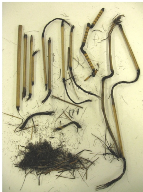
Figure 3 Remains of a Maori cloak and piu piu that has disintegrated in the iron-tannate dyed areas (Horniman Museum).
