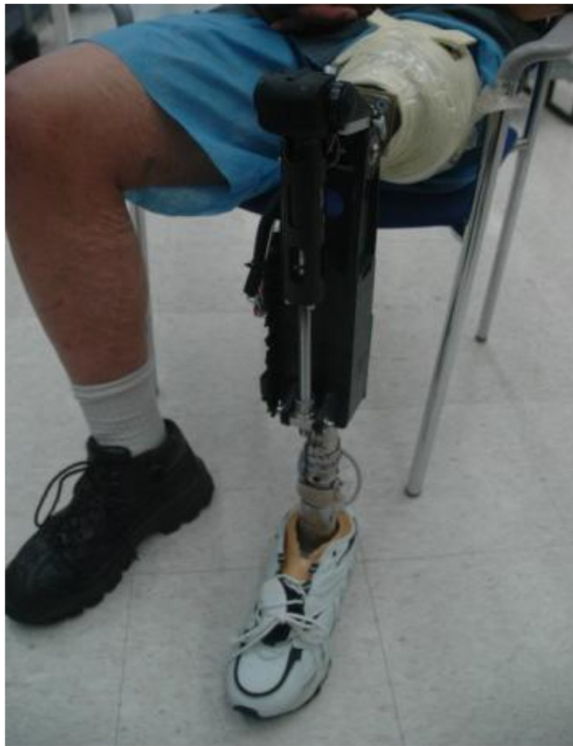
Figure 3 Transfemoral amputee wearing the powered knee prosthesis.
